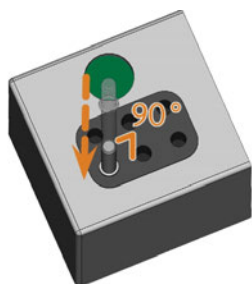
FIG. 43 – INSERTING TOOLS INTO THE TOOL POSITIONS
