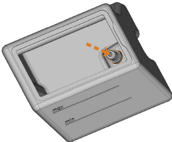
FIG. 90 – PUSHING THE COUPLING OUT OF THE TANK
