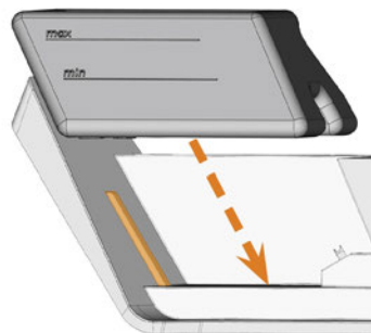
FIG. 38 – INSERTING THE COOLING LIQUID TANK INTO THE DRAWER (GUIDE RAIL COLORED ORANGE)
