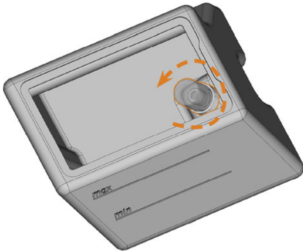
FIG. 89 – UNSCREWING THE FILTER IN THE COOLING LIQUID TANK
